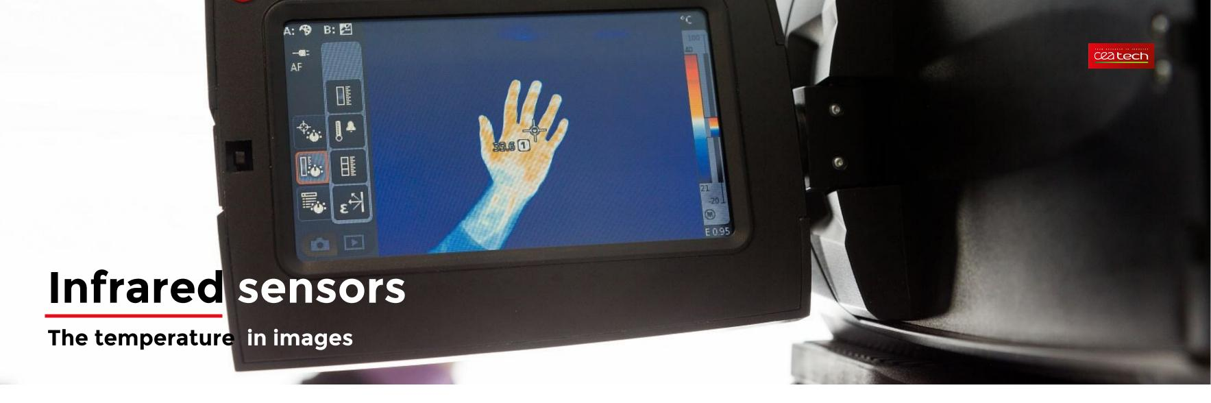
Until about 15 years ago, all infrared detectors were based on photodiodes and required cooling to around – 200 °C, making them very expensive.
